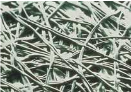
Figure 2: Typar® microscopic view
